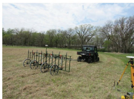
SENSYS MAGNETO MX V3 magnetic gradiometer in a 16-channel towed cart configuration.
